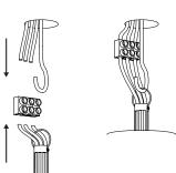
Connect the wires to the mains after setting up the hook.
